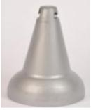
The V-Lock is Manufactured out of high grade A356, T-6 Grade Aluminum. With Precision we machine out the special cuts to allow the wrench to fall into place with the V-Lock this is done by CNC. Our Wrench Head is made out of the same material and requires more time for machining due to the reversed aspect of the cut to match the special fitting for adapting the V-Lock to latch in place and be able to be placed and removed on demand. Our Products are Made in the US!
